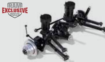
**3500 THE AVAILABLE AUTO-LEVEL REAR AIR SUSPENSION SYSTEM** deploys engineering specific to the weight class and the typically tougher assignments given to these pickups. Here, leaf springs are augmented with air springs mounted on top of the axle, resulting in the air springs and leaf springs working together for load carrying. The technology is utilized in both 2015 Ram 3500 single-rear-wheel and Dually models.
