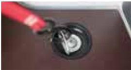
Its dual design addresses convenience and cargo protection. The standard load floor offers up to ten steel tie-down rings, each rated at 1,000 lb; cargo remains secure. Additional rings in the walls and partitions can bring the total up to 17 rings in all. Pre-cut holes in the available resin-finished wood load floor guarantee easy access to every floor ring.
