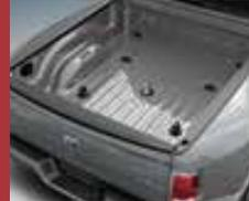
Available frame-mounted Gooseneck Hitch Ball from Mopar features easy ball removal when you need a flat bed. Optional Fifth-Wheel/Gooseneck Prep Package also includes in-bed 7-pin connector. (Ball not included in Packages.)
