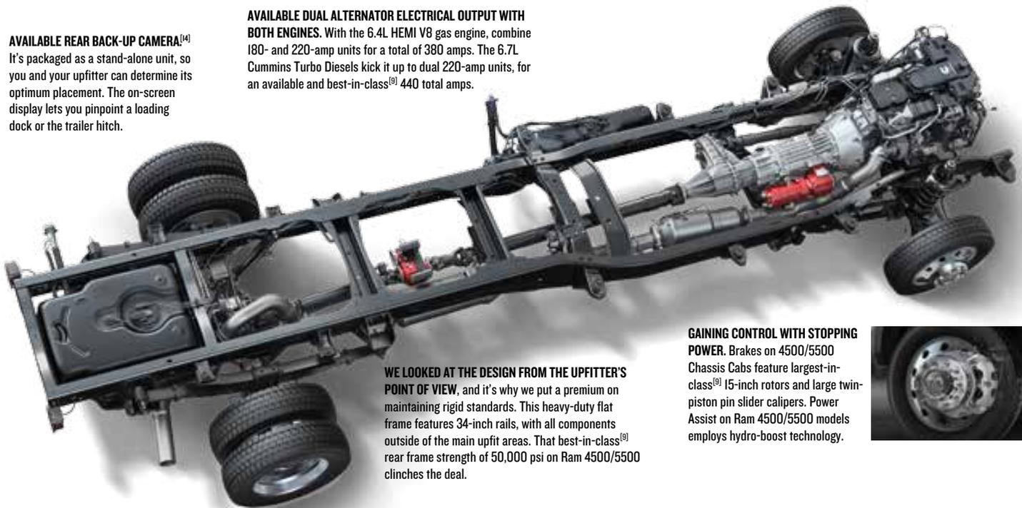
**WE LOOKED AT THE DESIGN FROM THE UPFITTER'S POINT OF VIEW,** and it's why we put a premium on maintaining rigid standards. This heavy-duty flat frame features 34-inch rails, with all components outside of the main upfit areas. That best-in-class<sup>[9]</sup> rear frame strength of 50,000 psi on Ram 4500/5500 clinches the deal.
